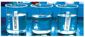
Water and chemical resistant: glass plates with laminated labels attached were immersed in water and various chemicals for two hours. The text was unaffected
